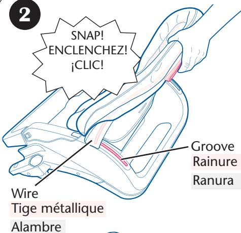
Squeeze recline handle and guide wire into groove.
